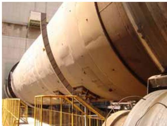
The gases released as part of the aerobic digestion is fired in the main firing. The material, after a residence time and aerobic digestion for 3 days, is fed in the calciner or kiln inlet.
