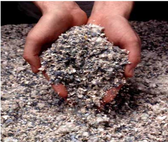
cement industry. At Castle Cement, tires are both fed as whole tires at the kiln inlet or shredded into chips and fired in Calciner. This waste not only comes with a significantly good calorific value but also with a good gate fee.
